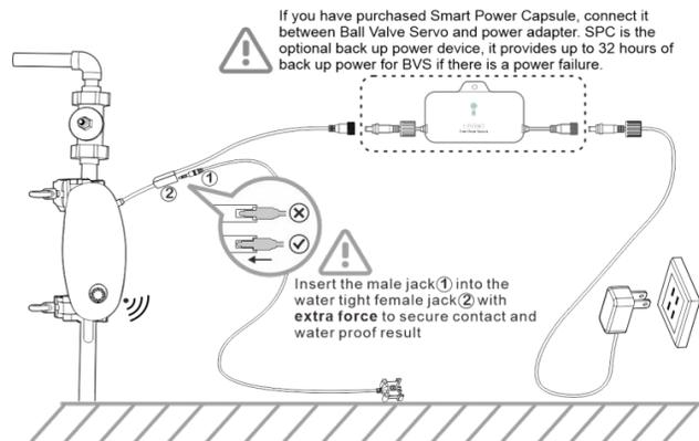
If you have purchased Smart Power Capsule, connect it between Ball Valve Servo and power adapter. SPC is the optional back up power device, it provides up to 32 hours of back up power for BVS if there is a power failure.
