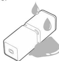
Put WWD on flat solid surface, drop water on it's side, let the water goes in to the groove underneath until water tripped 2 probes
